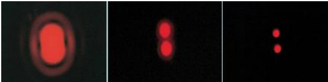
Fig. 32: The same object observed from three different telescopes with increasing diameter of the objective (from left to right). We see that increasing diameter of the objective improves our angular resolution.
